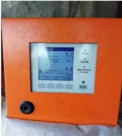
Sick Opacity meter in all stacks
